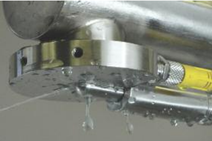
Dosing valve shut
